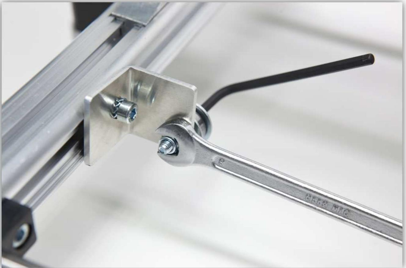
As you look from the bottom, the X BELT CLAMPS and the X pulley should be in one line. Slide the X PULLEY BRACKET until it is in one line with the two X BELT CLAMPS and then tighten the bolt holding it to the base frame. **Make sure it is perfectly horizontal.**
