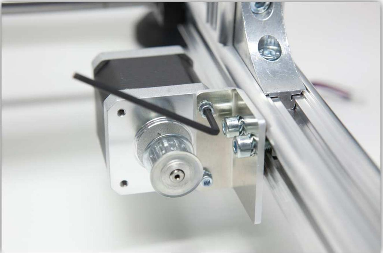
The pulley of the motor should be in line with the 2 X BELT CLAMP pieces. Slide it in place and tighten the bolts. **Make sure it is completely level.**
