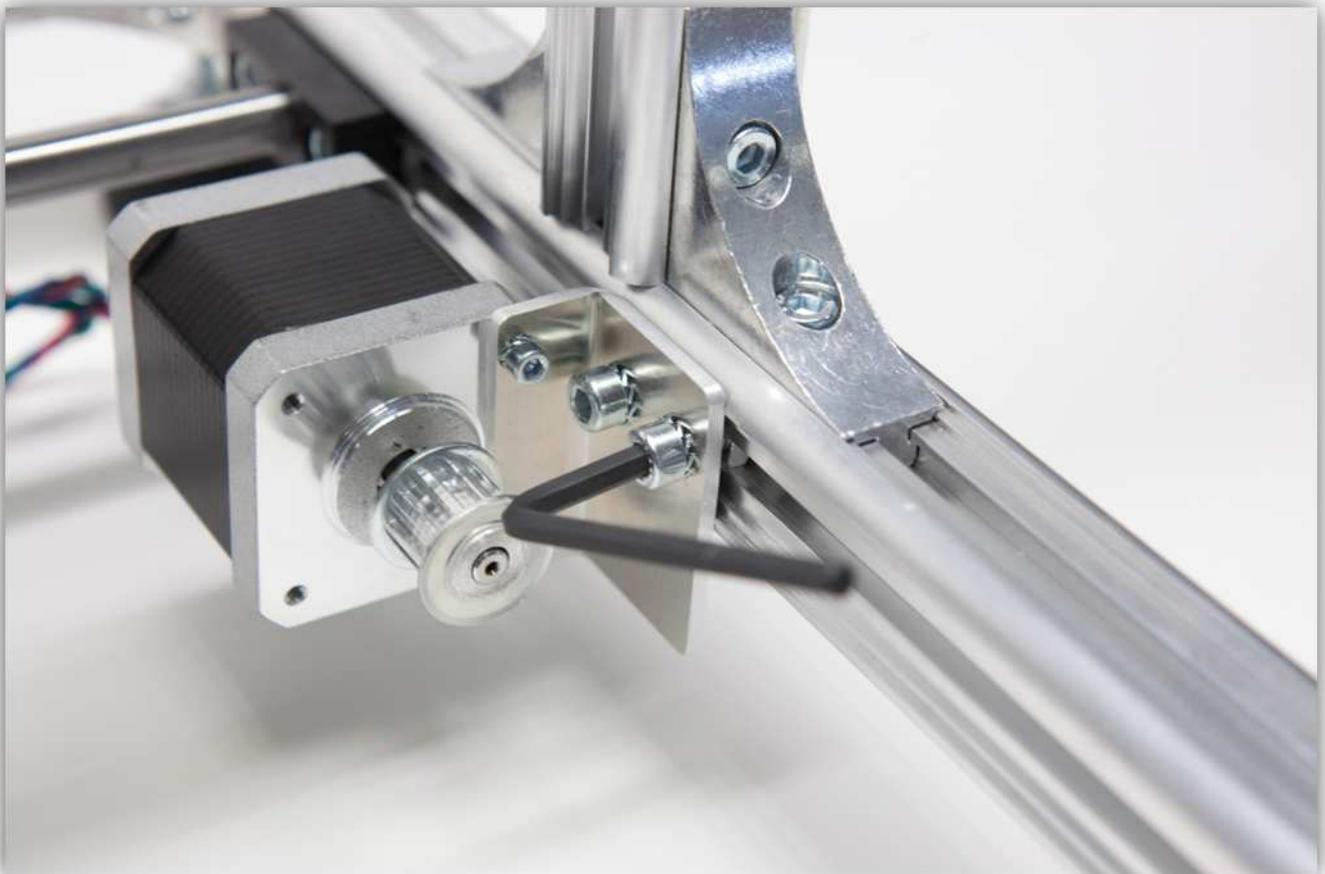
Now clamp the end of the belt into the leftmost X BELT CLAMP. Tighten the nuts.
