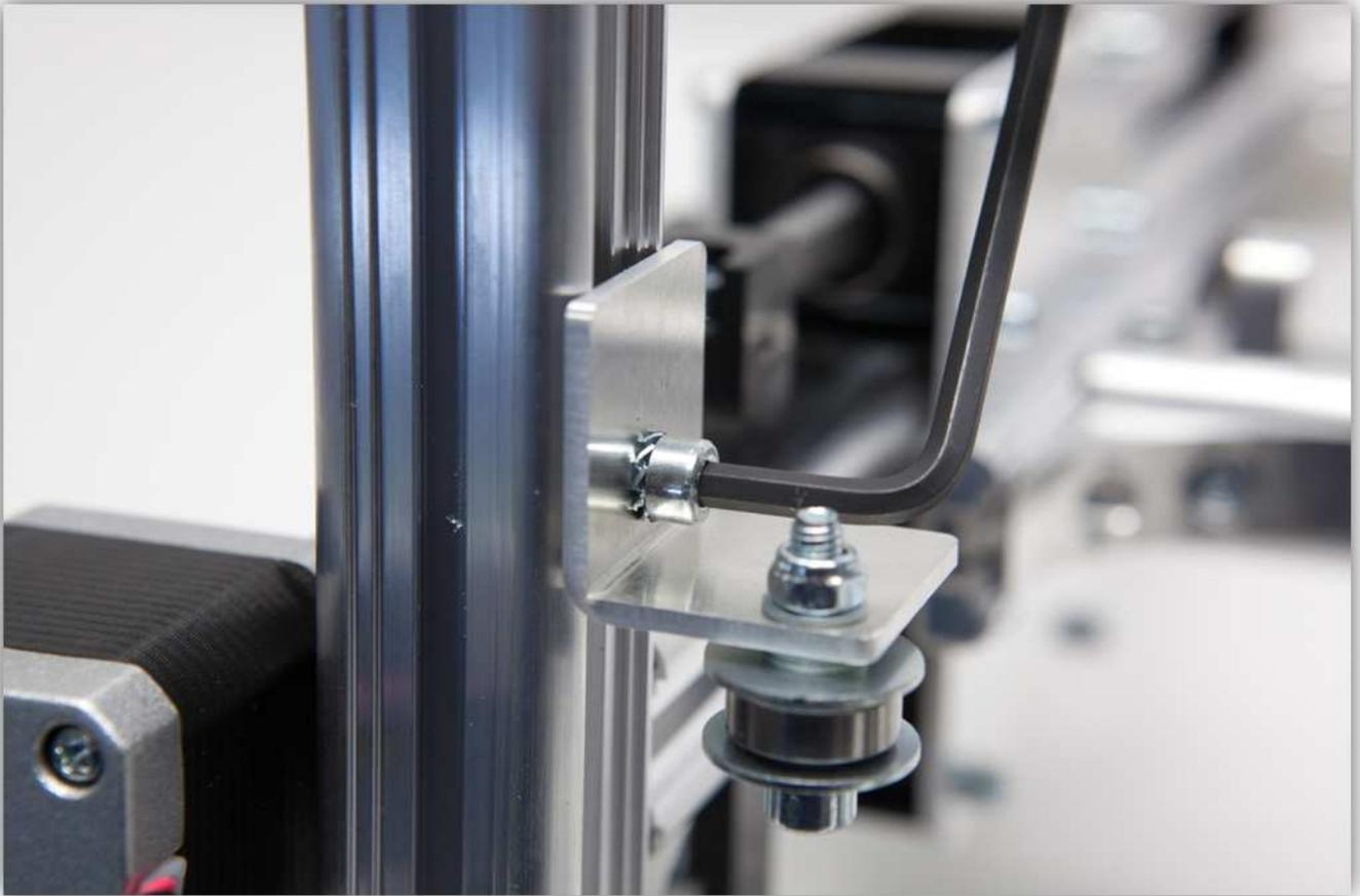
Take two short M5 bolts and two M5 toothed washers and screw the X MOTOR BRACKET to the 2 square nuts on the right side of the base frame you put there earlier. **Do not fully tighten the bolts.**
